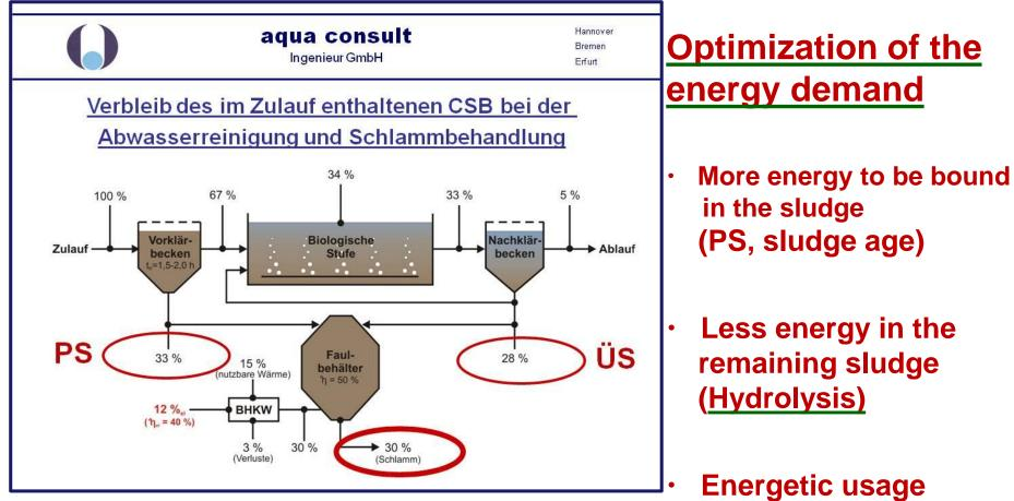
Energetic usage (Degasification, Hydrothermal treatment?) Energy-Balances for WWTP's
