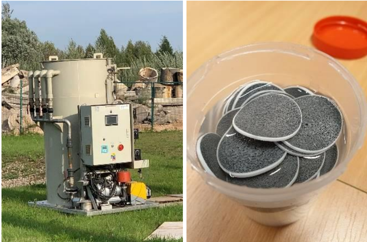
Figure 1. Picture of the pilot-scale MBBR at the territory of “Latvijas Piens” Ltd (A); carriers for biomass in MBBR (B).
