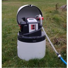
To increase the wastewater monitoring capacity at the Põltsamaa MWWTP, a portable automatic water sampler was purchased. As the sampler is portable, it can be used for monitoring wastewater in the entire catchment area. The sampler enables the MWWTP to monitor its customers wastewater discharges with increased reliability in situ, which helps the MWWTP in achieving better and more efficient process control.
