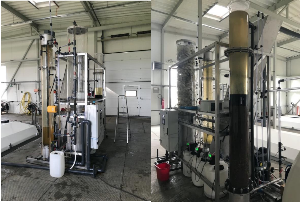
Figure 3. The test rig for tertiary wastewater treatment, built for and used in the project.
